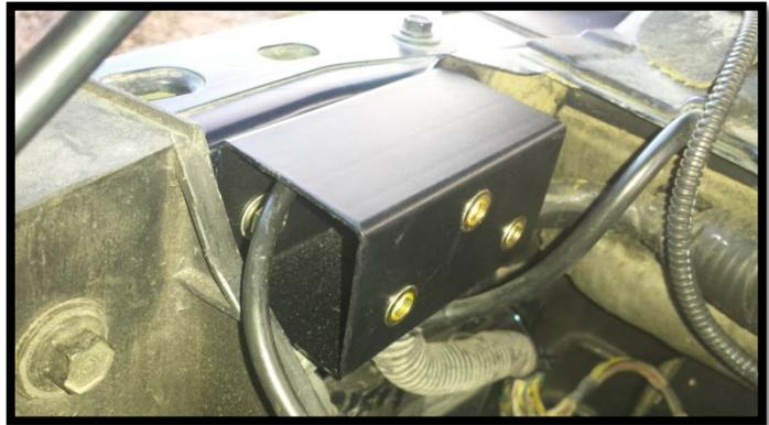
After the bracket is in place and tight all you have to do is mount the filter housing to it. I used stainless bolts and washer for everything to help with rust.
