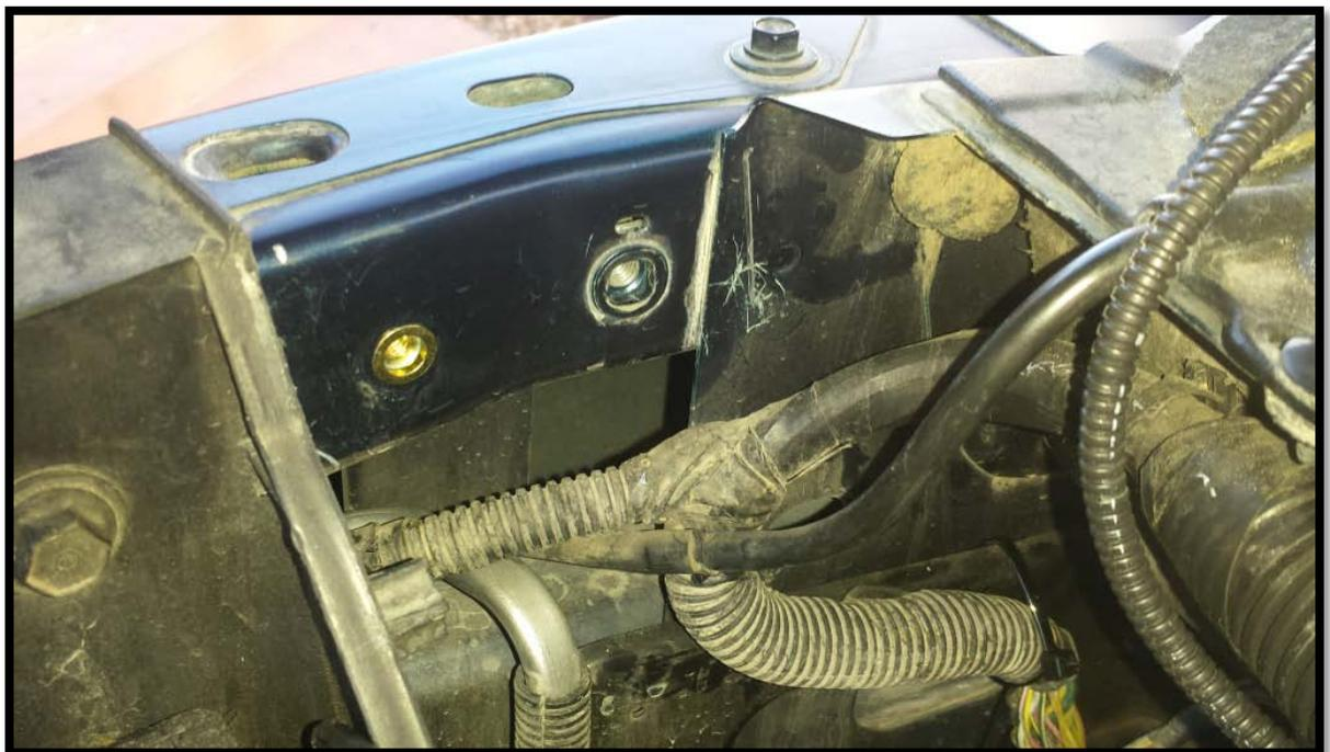
cable and the plastic clip that was right next to it, I went and drilled out the hole where the plastic clip was and added a 1/4x20 nutsert. These are very handy and make installs like this much more convenient as you don't have to worry about getting a nut on the backside of the bolt.
