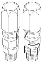
**Caution:** Do not introduce a twist to the hose when tightening the BP261 to the BP208 (or BP242).
